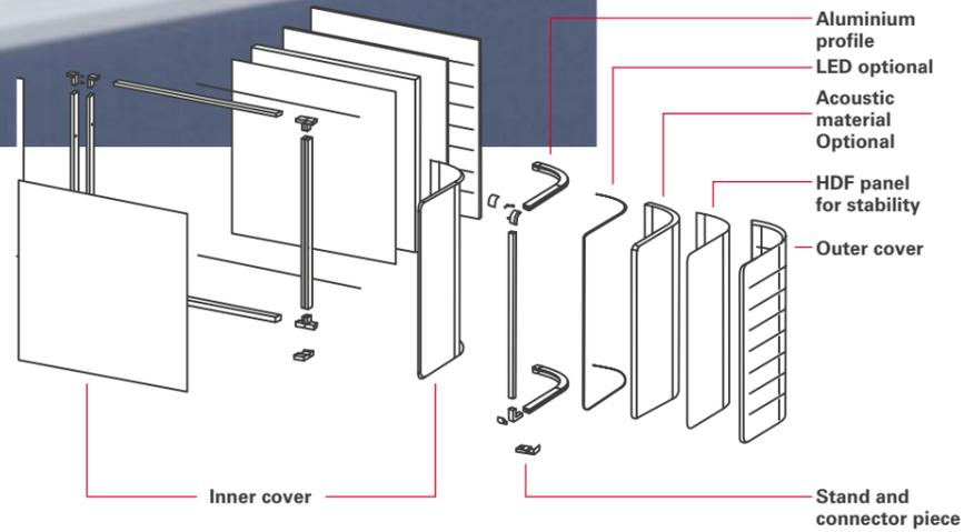
The innovative HUB screen wall comprises three elements: A left-hand and a right-hand curved element and a central section. The individual parts can be assembled using a click-on connection and detached again just as easily for compact storage. The **curved aluminium profile** is unique in its production, and makes the partition and backing screens particularly high-quality and stable.
